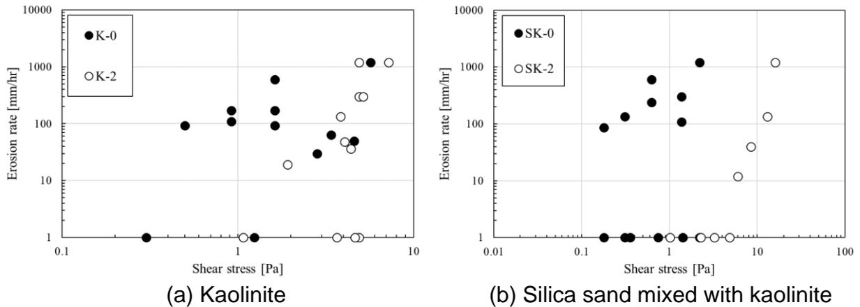
Fig.3 Effect of Xanthan gum content on the erosion resistance of different soils.
