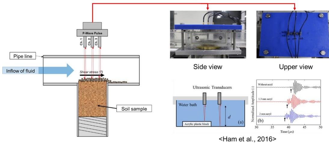
Fig. 1 EFA set-up
